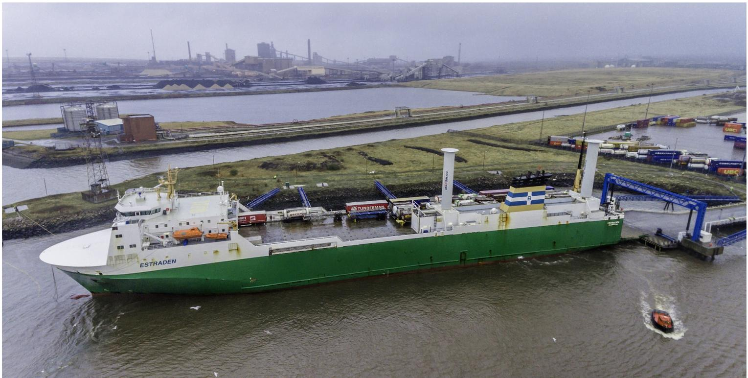
Spinning cylindrical sails can be used on large ships to reduce greenhouse gas emissions and propel them forward. Image credit - Norsepower
